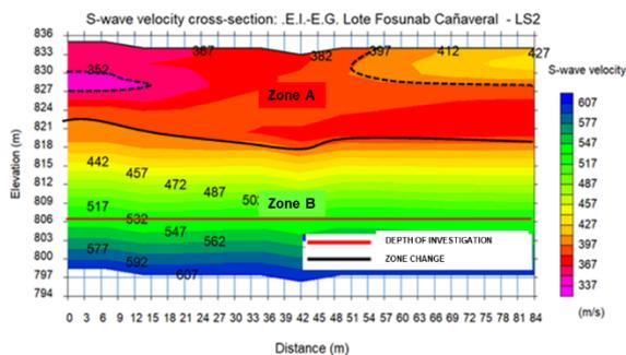
**Figure 4.** MASW/2D LS2 Surface Wave Testing.
