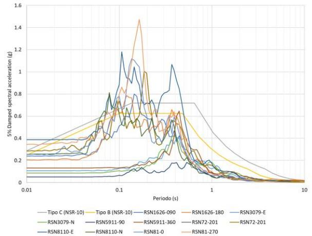
**Figure 13.** Spectral accelerations obtained at the surface.
