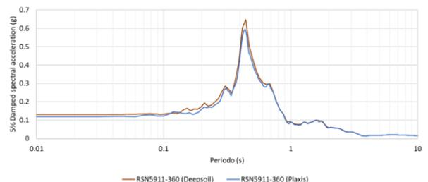
**Figure 14.** Surface response spectrum Deepsoil-plaxis signal RSN5911-360.
