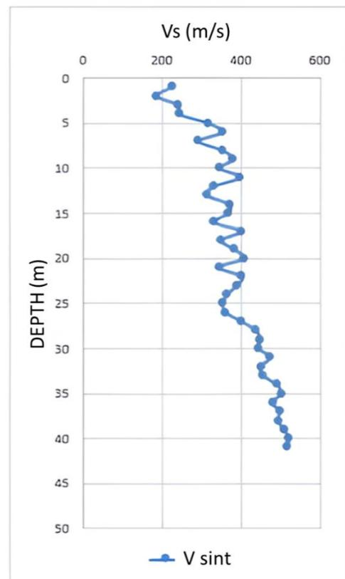
**Figure 5.** Vs intervalic: Down Hole Test
