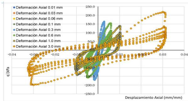
Figure 6. Cyclic triaxial test (400 kPa)
