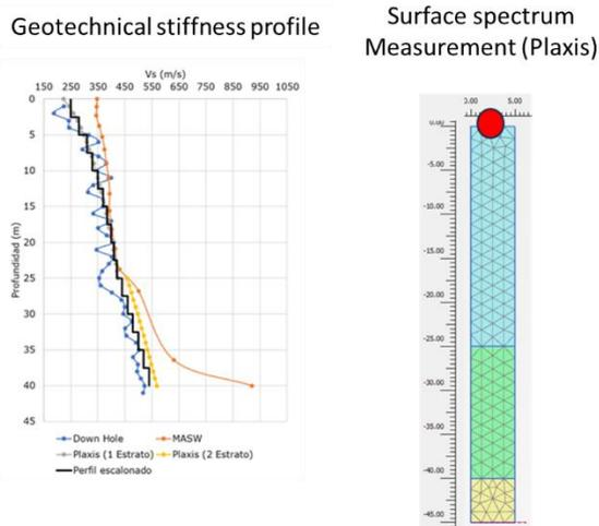
**Figure 12.** Geotechnical low strain stiffness profile and plaxis surface response modeling.
