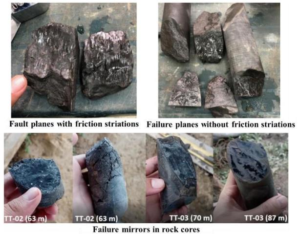
Figure 5. Cutting surfaces cores found.
